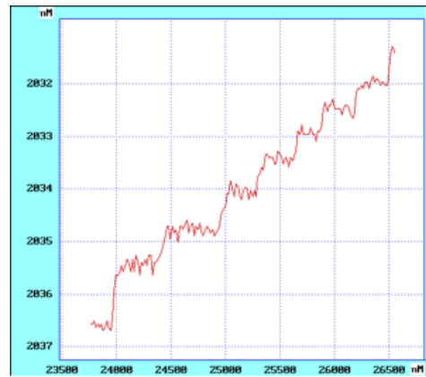
Graduated surface of basic sapphire surface (c-plane), and its section by the given plane. Graduated surface is obtained by annealing the sample at the 1350 °C.
